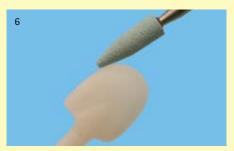
Accurate finishing in the shoulder area with the fine Diagen-Turbo-Grinder for precise restorations made of press ceramic, layering ceramic or zirconium. A perfect surface for subsequent polishing with Zi-polish is obtained.
