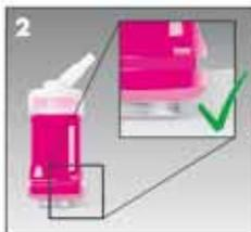
**Immediately** start mixing for 15 seconds at 4000-4500 osc./min.
